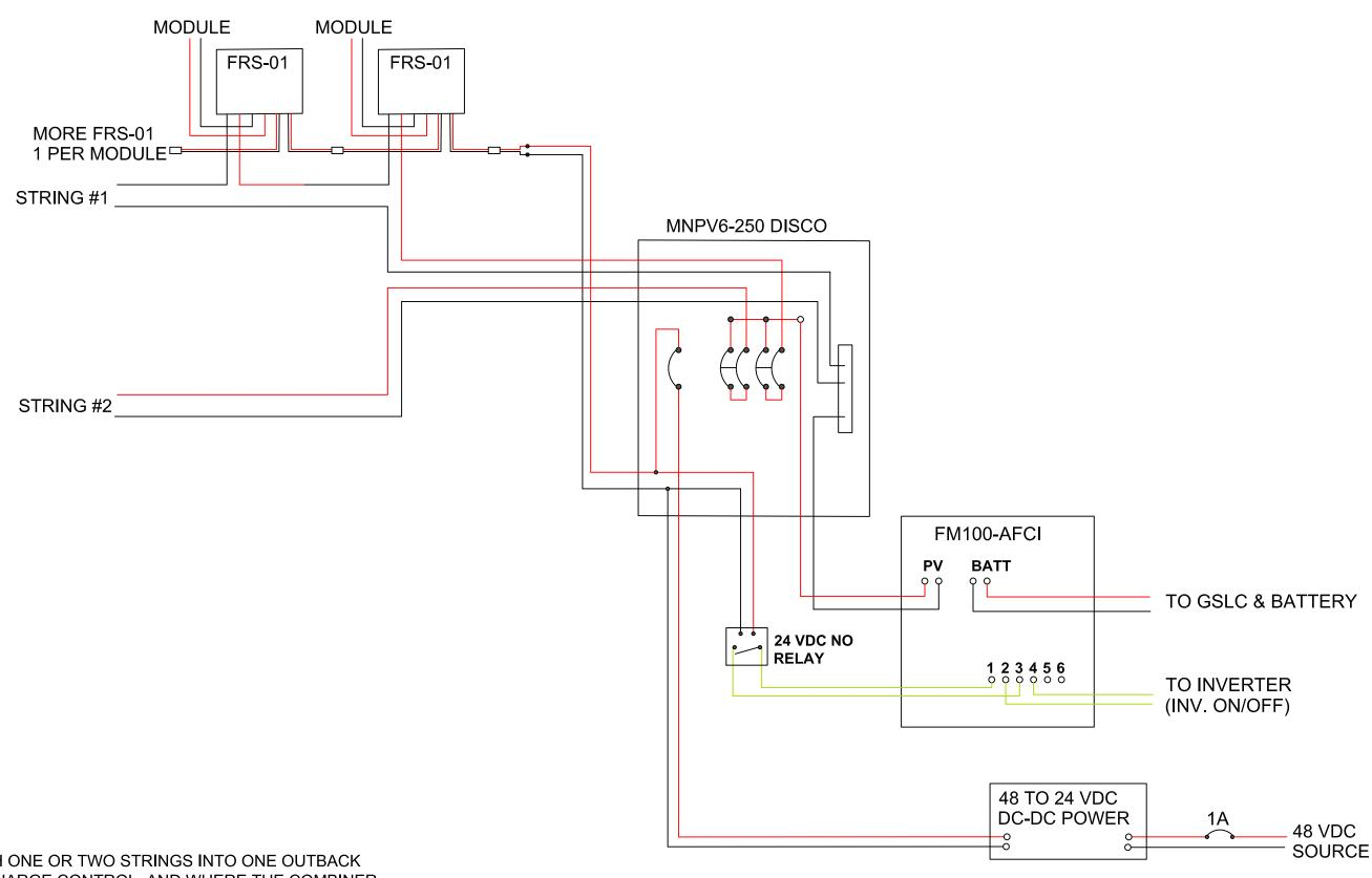
FOR USE WITH ONE OR TWO STRINGS INTO ONE OUTBACK FM100-AFCI CHARGE CONTROL, AND WHERE THE COMBINER CAN BE PLACED WHERE IT IS NEEDED FOR RSD
