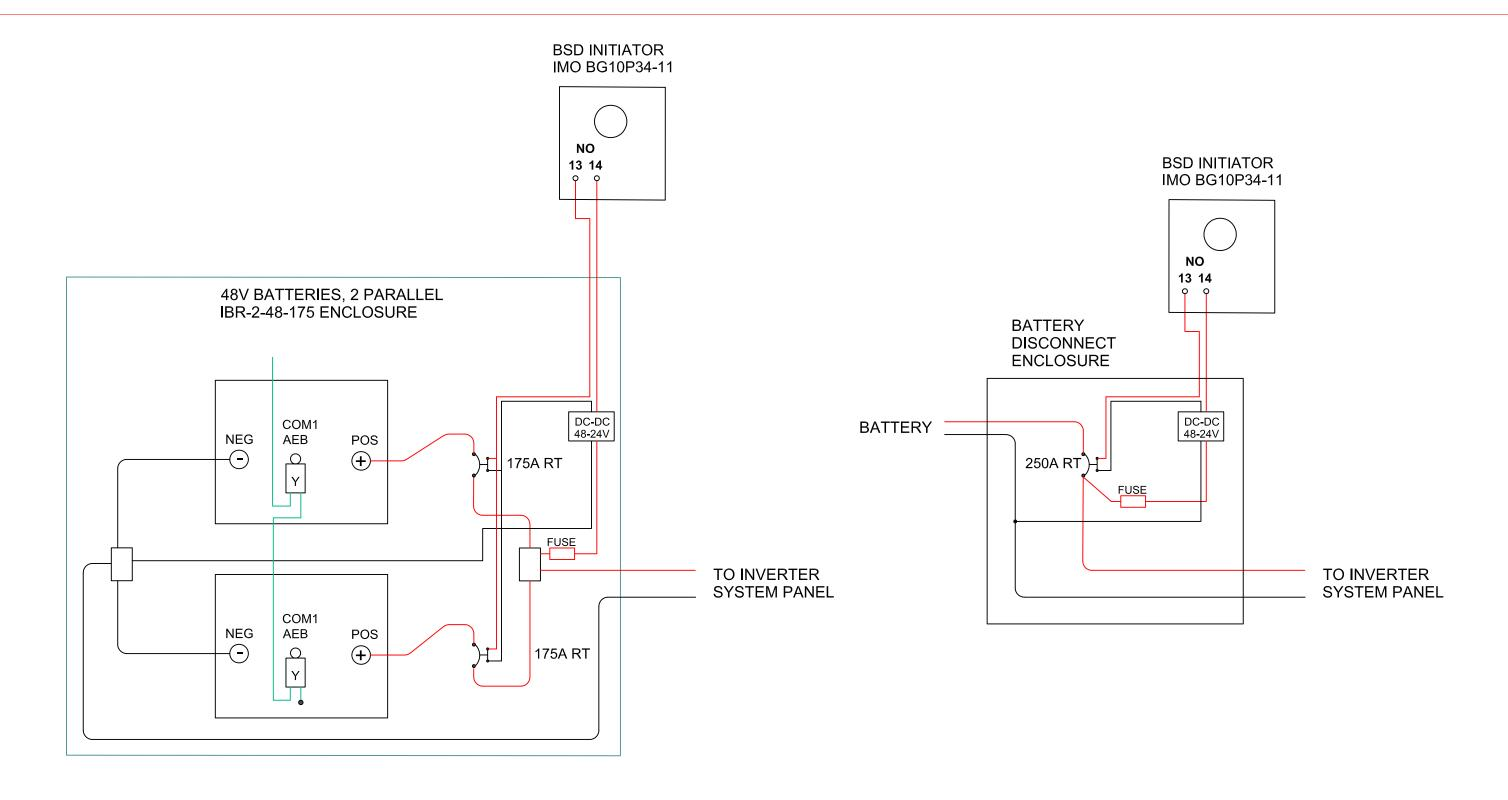
NOTE: THIS MUST BE ARRANGED SO THAT WHEN THE INITIATION DEVICES IS CLOSED FOR BATTERY SHUTDOWN, THE POWER TO THE CONTROL CIRCUIT MUST ALSO BE INTERRUPTED WHEN THE BATTERY BREAKERS OPEN. THIS IS TO PREVENT THE COIL IN THE REMOTE BREAKER(S) FROM HAVING CONTINUOUS POWER TO IT WHICH WILL BURN IT OUT.
