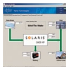
The Solaris RS-232 interface shows graphically what power is being produced and where it is going (grid-tie shown).
